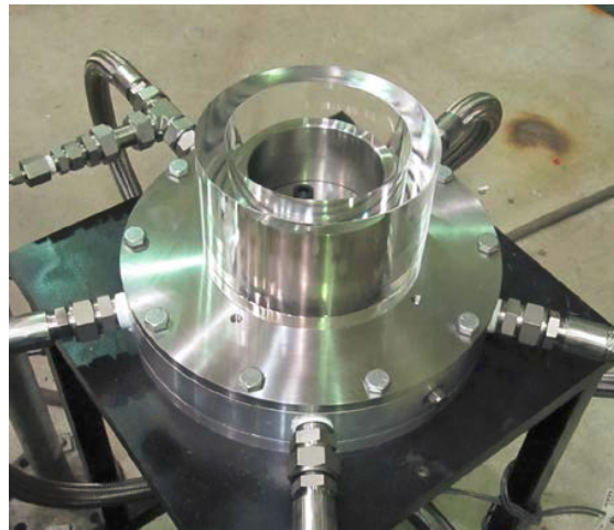
Figure 2.1: RDE with quartz outer body to allow visualization of the flow field inside of the RDE [9].
